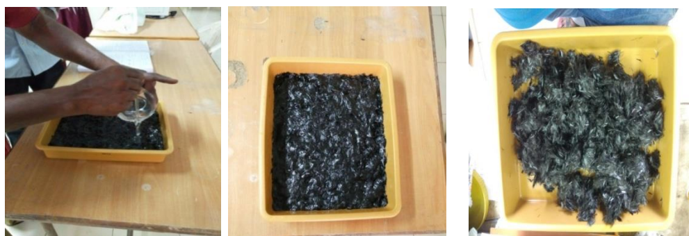
Fig 2.4.1 Sequence of operations in Acid HNO 3 Treatment on CF and GF surface
